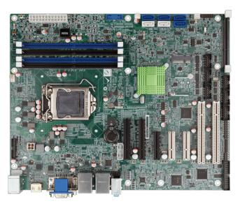
ATX motherboard supports 14nm LGA1151 Intel® CPU Intel® Q170,
