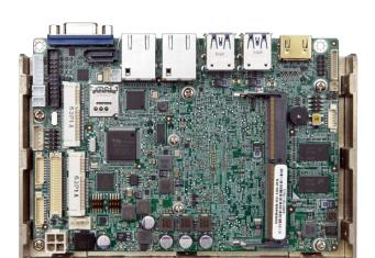
3.5" SBC supports Intel® 6th Generation ULT Processor with DDR4 SO-DIMM/On-board Memory Support
