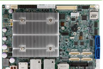
3.5" SBC supports Intel® 14nm Generation Atom™ or Celeron® on-board SoC with DP++/VGA/LVDS/iDP support
