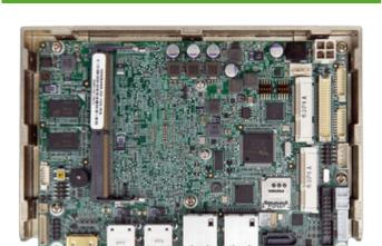
3.5" SBC supports Intel® 7th Generation ULT Processor with DDR4 SO-DIMM/On-board Memory Support
